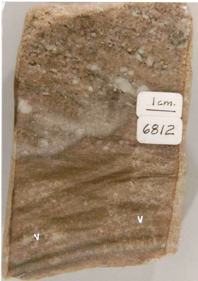
FIG. 25b— Narrow hori- zontal and vertical bands of tightly-cemented sandstone forming a lattice pattern (arrows). Depth in feet.
