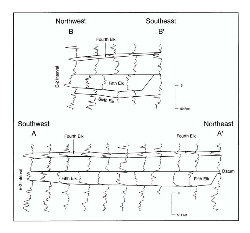
Figure Des-34b. Gamma-ray log cross sections across Council Run field. The geometry of the Fifth Elk suggests a fluvial point-bar deposit. See Figure Des-34a for location of cross sections.
