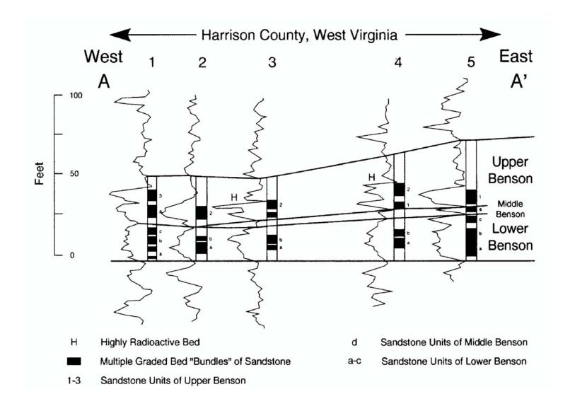
Figure Des-20b. Cross section of the Benson interval including the highly radioactive bed. See Figure Des-17a for location of cross section.
