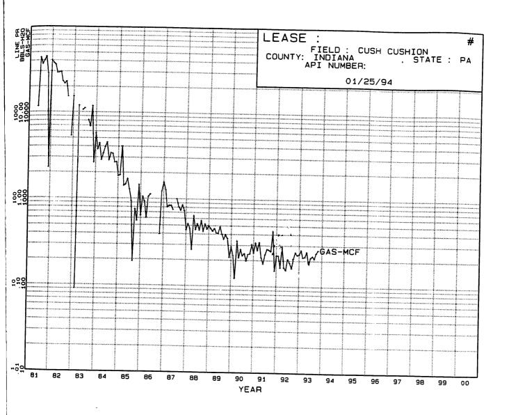
Figure 5. Gas production decline curve from a well in the Cush Cushion field. Monthly and yearly production is presented from the turn in line date (June 1981)through late 1993.
