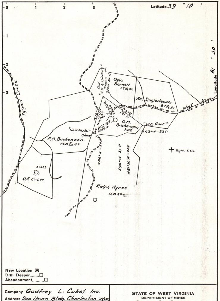
Address 900 Union Blog. Charleston Wva. Farm Sarah E. Single decker GLC 086 Well (Farm) No. / Serial No. /345 Elevation (Spirit Level) 885.72 Quadrangle Belleville County Wood A District Steele Engineer's Registration No. \_ \_\_Drawing No. Date /2-/6-50 Scale / = /320'
