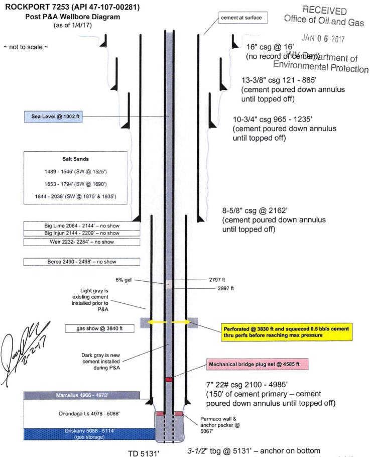
(total of 703 bags of cement "poured" down 3-1/2" x 8-5/8" annulus in 6 trips to well)
