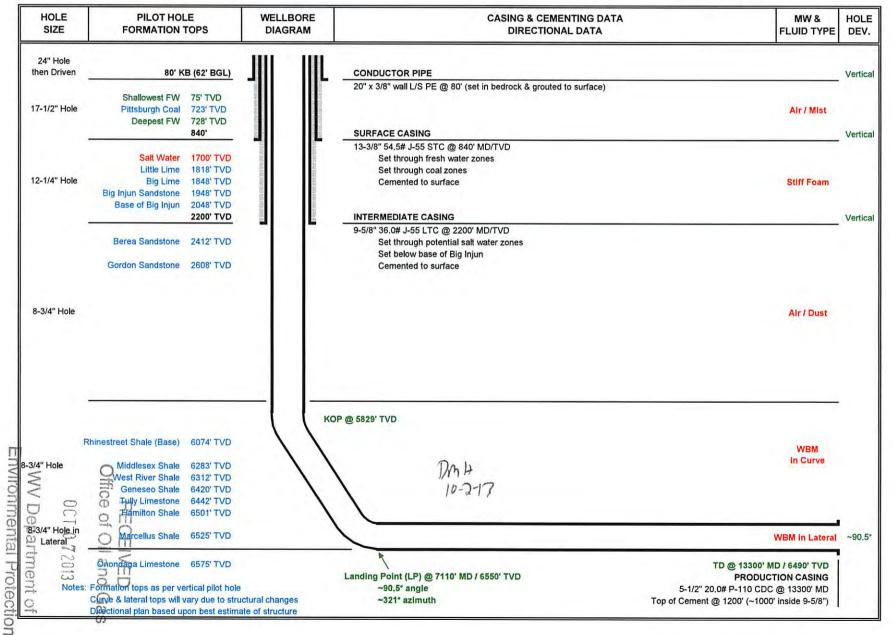
NOTE: THIS DRAWING IS NOT TO SCALE. THE DIMENSIONS REFLECTED ON THE DRAWING ARE ESTIMATED MEASUREMENTS AND FOR 4710302946 24.25" 19.25" 2-1/16" API 5,000 2-1/16" API 5,000 38.26" 22.12" 2-1/16" API 5,000 5-1/8" API 10,000 19.50 1-13/16" API 10,000 5-1/8" API 10,000 13.25 11" API 5,000 feet 19.38" 2" API LINE PIPE 5.00" I.D. WELD PREP 9-5/8" SOW 9-5/8" RECEIVED Office of Oil and Gas
