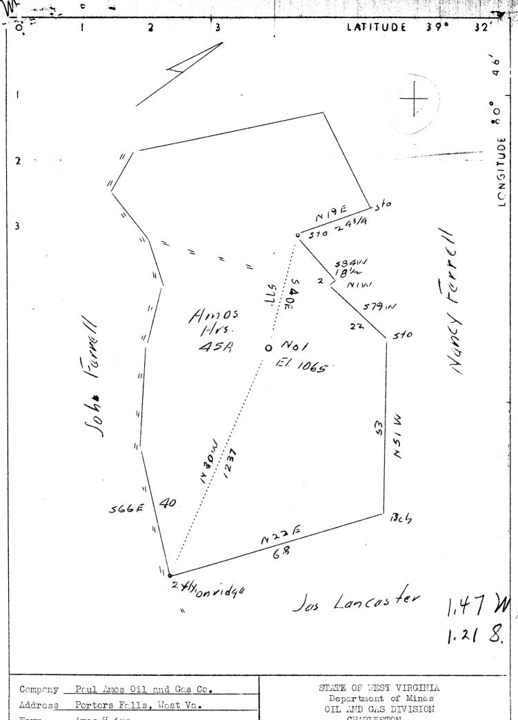
Amos Heirs Tract 1 Acres 45 Lease No. Well (Farm) No. 1 Serial No. Elevation (Spirit Level) Quadrangle New Martinsville County Wetzel District Green Engincor J.M. Cochran Engineer's Registration No. Co. Surveyor File No. \_Drawing N<sub>o•</sub> Date Oct. 6,1937 Scale 1"-330'
