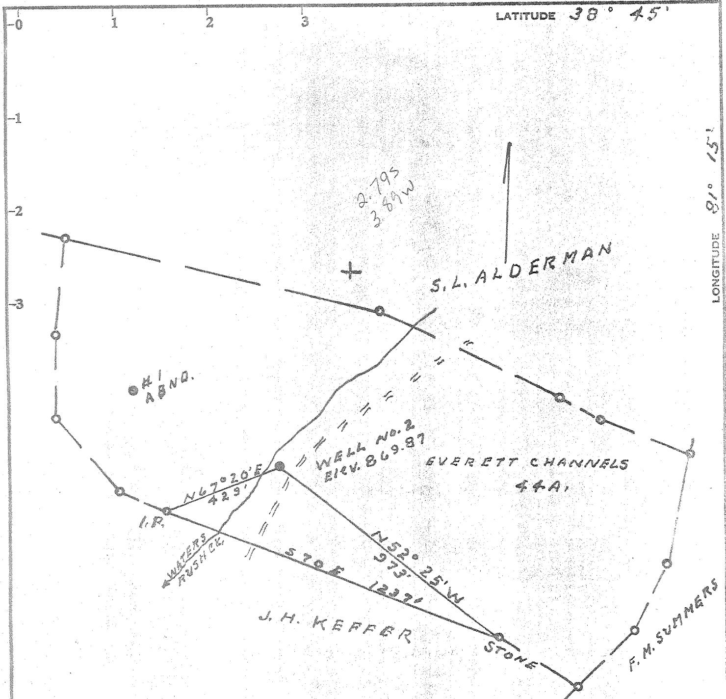
Minimum Error of Closure 11 IN 200'Source of Elevation FORKS ROAD SOUTH 810.00Fracture
