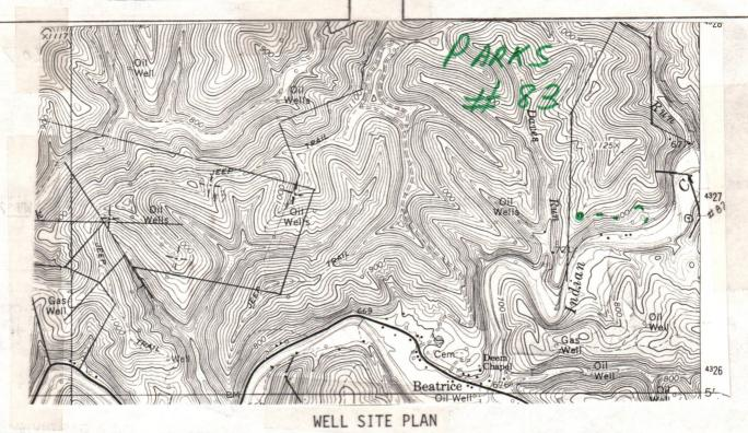
Sketch to include well location, existing access road, roads to be constructed, well-site, drilling pits and necessary structures numbered or lettrered to correspond with the first part of this plan. Include all natural drainage.
