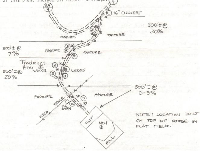
Access road subject to change between company and land owner, or aquirement of right-of-way. If change is made, a revised reclamation plan will be submitted. All cuts 2:1 slope. All topsoil to be stockpiled and used in reclamation. All grades for roads and locations as well as sediment structures shown on drawing.
