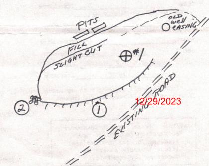
TREES TO BE CUT AND STACKED. BRUSH TO BE DISPOSED OF BEFORE EARTHWORK BEGINS. REVEGETATION TO BE COMPLETED WITHIN SIX MONTHS OF WELL COMPLETION.
