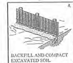
STAPLE WIRE FENCING TO THE POSTS
