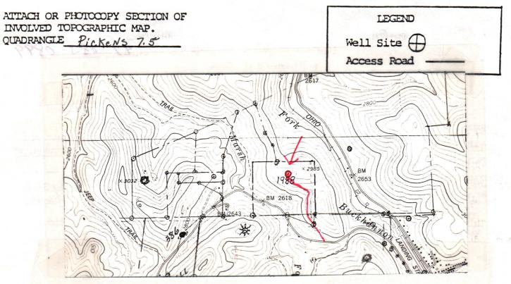
ketch to include well location, existing access road, roads to be constructed, wellsite, drilling pits and necessary structures numbered or lettered to correspond with the first part of this plan. Include all natural drainage.
