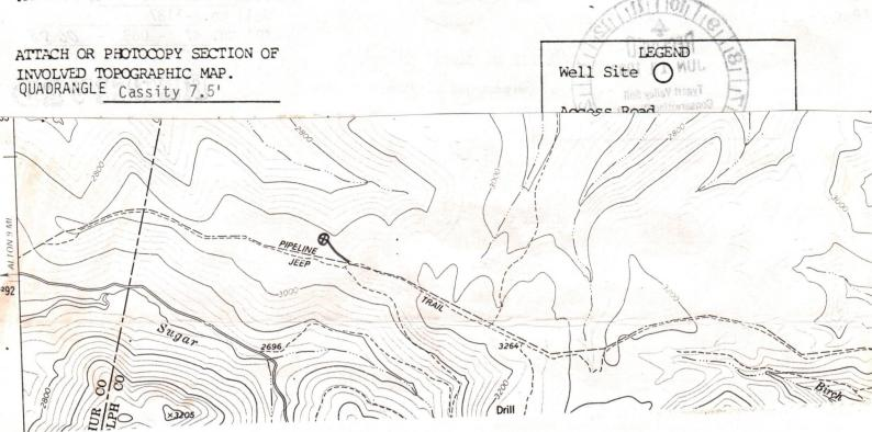
Sketch to include well location, existing access road, roads to be constructed, wellsite, drilling pits and necessary structures numbered or lettered to correspond with the first part of this plan. Include all natural drainage.
