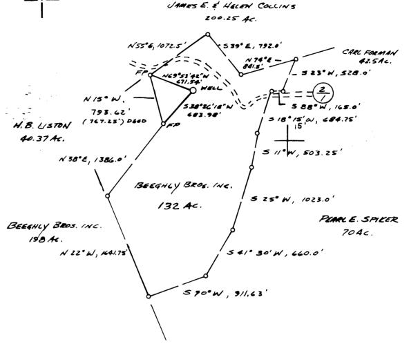
FILE NO .. DRAWING NO .\_ 1" = 1000" SCALE\_ MINIMUM DEGREE OF 1 IN 200 ACCURACY\_ PROVEN SOURCE OF ELEVATION BM - MOUNTAIN GROVE CHURCH EL. 1891
