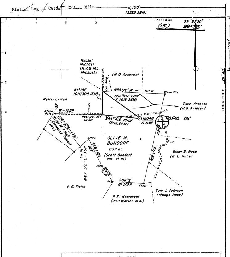
Minimum Error of Closure 1' In 200' Source of Elevation B.M. - Angle In Road Valley Point 7 1/2' Topographic Map
