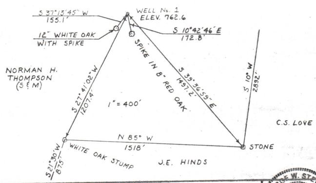
FILE NO .. DRAWING NO ... SCALE 1" = 400' MINIMUM DEGREE OF ACCURACY 1:200 PROVEN SOURCE OF ELEVATION\_U.S.G 1956 80 WSM
