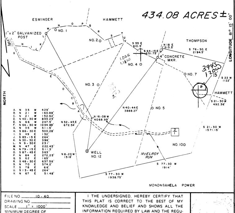
MINIMUM DEGREE OF ACCURACY ... 1/200 PROVEN SOURCE OF ELEVATION T. B.M. MON-POWER ELEV. 826.61 CO.
