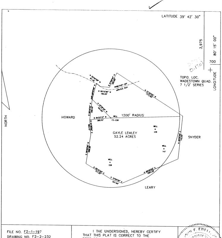
DRAWING NO. <u>F2-2-23</u>2 SCALE 1'' = 500'MINIMUM DEGREE OF ACCURACY 1/2500' PROVEN SOURCE OF ELEVATION \_ USGS B.M.
