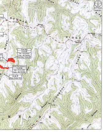
WV State Plane Coordinate System North Zone, NAD 83 Elevations Baxed on NAV88 Established By Survey Grade GPS and OPUS Post-Processing
