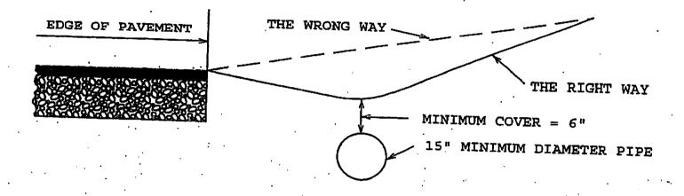
PIPE INSTALLATION FOR SIDE ROAD APPROACH WITH STEEP GRADE
