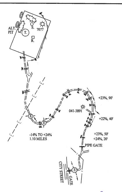
THIS PLAN IS FOR THE PLUGGING OF AN EXISTING GAS WELL. ENTIRE LENGTH OF ROAD IS OLD EXISTING WELL ROAD. ROCK WILL BE USED WHERE NECESSARY.
