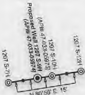
Wellhead Layout (NTS)
