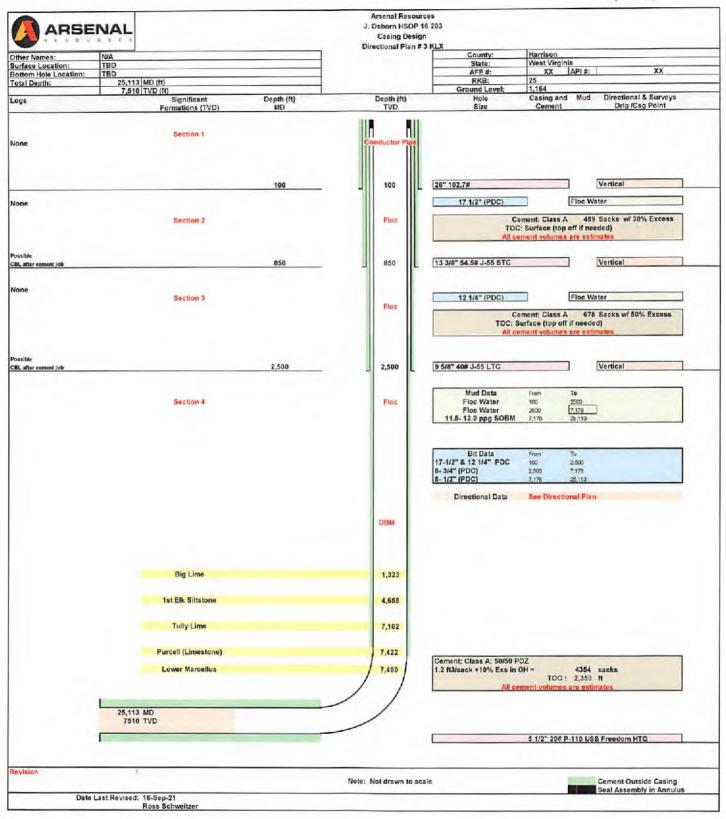
Area of Review Report - \_\_J Osborn HSOP16 \_\_\_\_ Pad, \_\_\_\_203 \_\_ Lateral, \_\_\_\_ Harrison \_\_\_ County, WV
