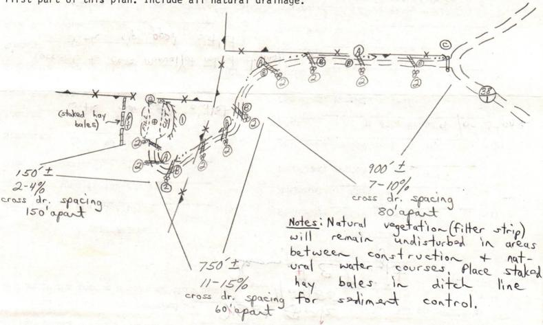
Access road subject to change between company and land owner, or aquirement of right-of-way. If change is made , a revised reclamation plan will be submitted. All cuts 2:1 slope. All topsoil to be stockpiled and used in reclamation. All grades for roads and locations as well as sediment structures shown on drawing.
