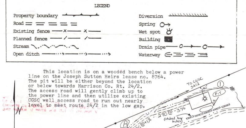
Timber will be cut and stacked and topsoil will be stockpiled for use in revegetation. An iron gate has been maintained at the junction of said well road with 24/2. Rock will where necessary. used on road Natural regetation (filter strip) Will in undisturbed areas remain between construction of natural courses. Place staked hay bales ditch line for sediment control in
