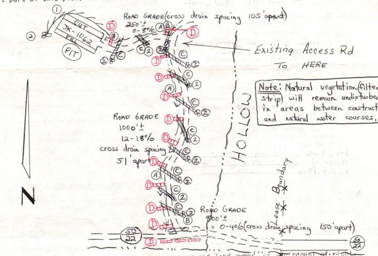
Access road subject to change between company and land owner, or attirement of right of-way. If change is made, a revised reclamation plan will be submitted. All cuts 2:1 slope. All topsoil to be stockpiled and used in reclamation. All grades for roads and locations as well as sediment structures shown on drawing.
