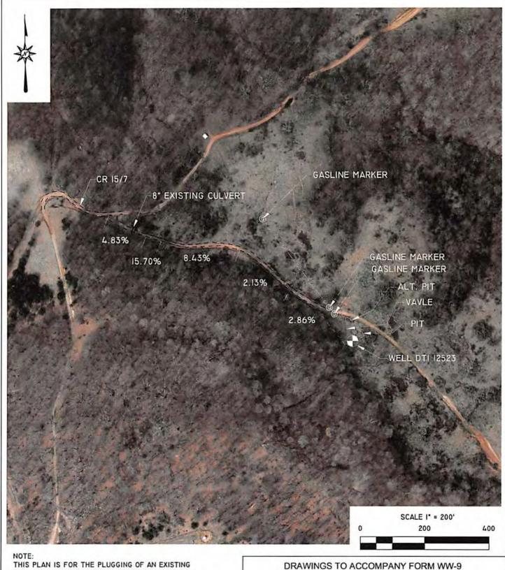
GAS WELL. ENTIRE LENGTH OF ROAD IS EXISTING ROCK BASE WELL ROAD. ROCK WILL BE USED WHERE NECESSARY. ALL GRADES ARE NOTED.
