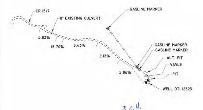
NOTE: THIS PLAN IS FOR THE PLUGGING OF AN EXISTING GAS WELL. ENTIRE LENGTH OF ROAD IS EXISTING ROCK BASE WELL ROAD. ROCK WILL BE USED WHERE NECESSARY. ALL GRADES ARE NOTED.
