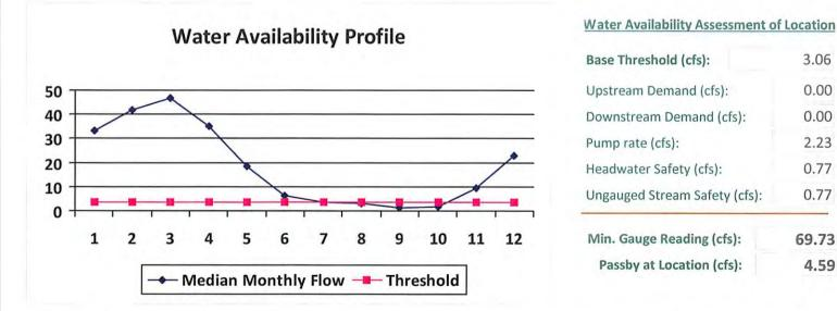
"Threshold", as depicted in the chart above is meant only to indicate the calculated base threshold at the proposed withdrawal location. This value does not include the proposed pump rate or existing demand on the stream. Refer to the monthly breakdown above for a more complete estimation of water availability by month.
