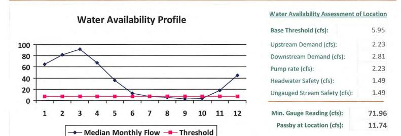
"Threshold", as depicted in the chart above is meant only to indicate the calculated base threshold at the proposed withdrawal location. This value does not include the proposed pump rate or existing demand on the stream. Refer to the monthly breakdown above for a more complete estimation of water availability by month.
