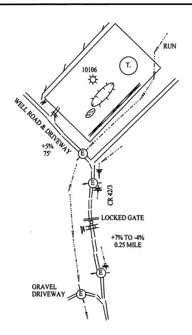
THIS PLAN IS FOR THE PLUGGING OF AN EXISTING WELL. ENTIRE LENGTH OF ROAD IS EXISTING COUNTY ROAD AND WELL ROAD. ROCK WILL BE USED WHERE NECESSARY.
