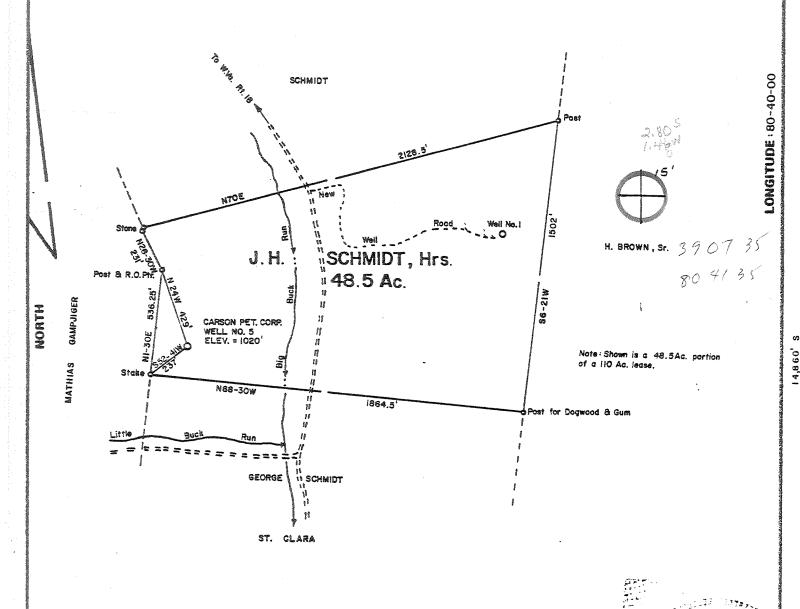
FILE NO. DRAWING NO .. SCALE \_\_ | inch = 500 feet MINIMUM DEGREE OF ACCURACY 1/200 PROVEN SOURCE OF ELEVATION U.S.G.S. BM 700 NE Location , Elev. = 877'
