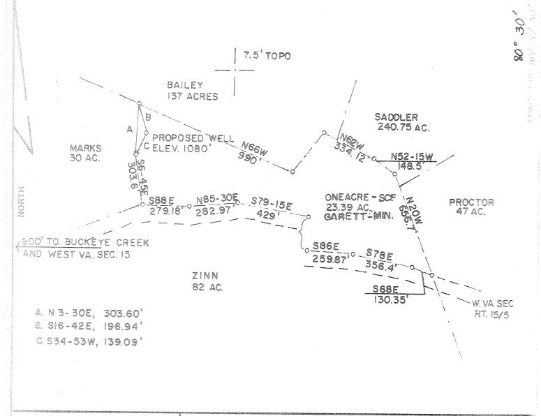
FILE NO .\_ DRAWING NO .. SCALE 1" = 400' MINIMUM DEGREE OF ACCURACY 1 IN 200 PROVEN SOURCE OF ELEVATION USGS BM ZINNIA 898 USGS BIG ISSACC QUAD
